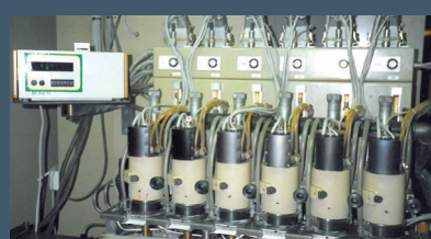
The 6-spindle NC machining centre CPW Cal.12
